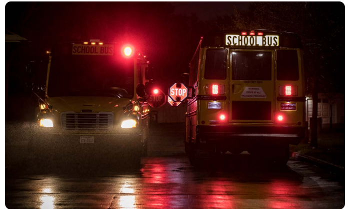
Comparison: traditional stop arm (left) vs. First Light’s fully illuminated stop arm (right) in low light
