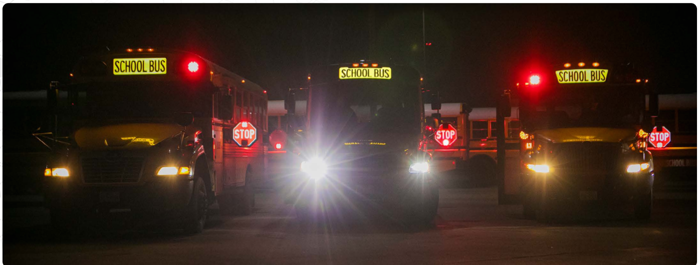
Increased visibility in low light conditions by fully illuminating the stop octagon
