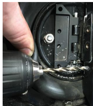
FIGURE 6: Drilling first hole to mount new hinge
