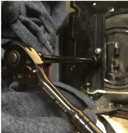
FIGURE 5: Removing hinge screws and aligning new hinge
