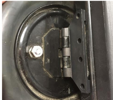
FIGURE 5: Removing hinge screws and aligning new hinge
