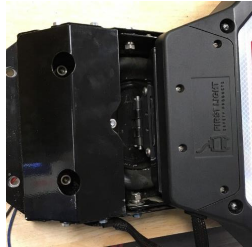
FIGURE 11: Reinstalled cover on stop arm with new hinge
