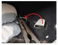
b. Unhook the other end of the spring from the wire rope lug.
