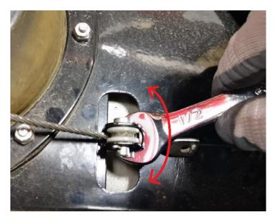
b. Remove the pulley wheel & clevis pin by pulling out the cotter pin with pliers:
