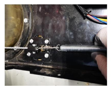
b. Using the same method as in step 2, reattach the other end of the spring to the base tab.
